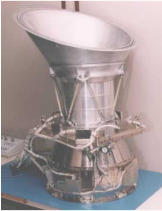
Fig. 1. The long conical radiators of the MOS enable the radiating surface to reach the plane of the spacecraft thermal shield to avoid parasitic heat-loads.
